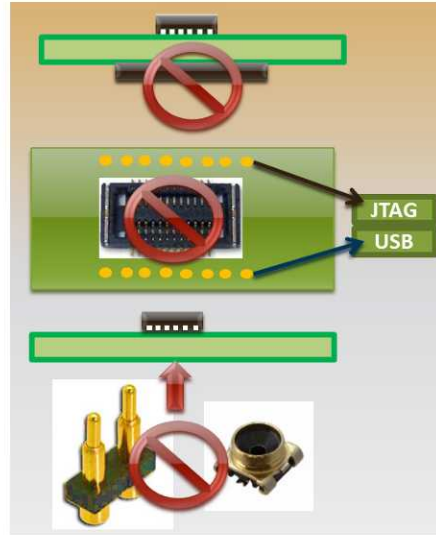
Figure 2. Avoid connectors directly behind the board
